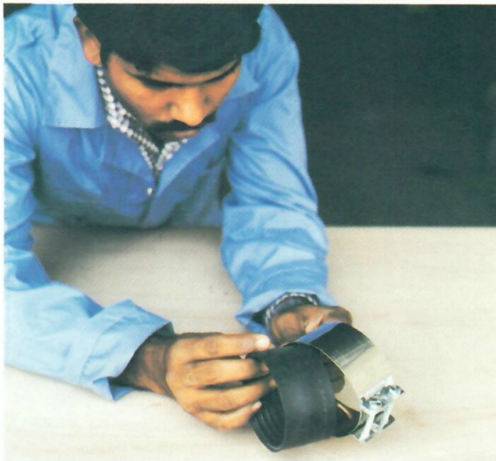
Step 1 – Separate rubber seal from steel fastener
